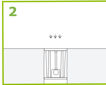
Insert a sleeve into a hole
